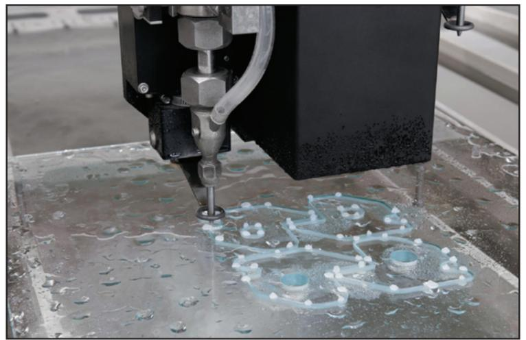
The machine has quick and precise height sensing with low sensing pressure, integrated collision monitoring, and automatic nozzle calibration.
